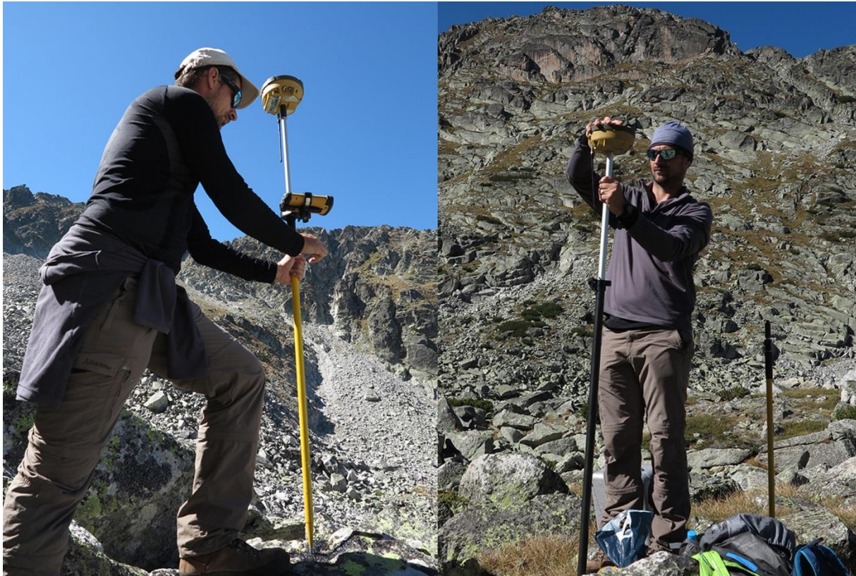
Fig. 5. Ground based geodetic measurements using a differential GPS.
