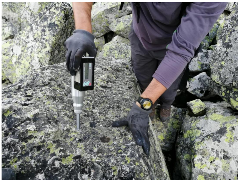
Fig. 3. Using Schmidt hammer on M4 rock glacier in Rila Mountains.
